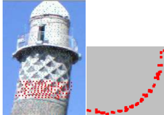
Figure (6) Scanned points superimposed on the harsh engravings around the surface of the trunk.
