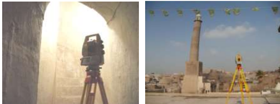
Figure (2) Topcon Imaging Station at work inside and outside the minaret.
