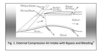
Figure (1) External Compression Air Intake with Bypass and Bleeding<sup>4</sup>.
