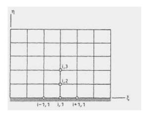
Figure (3) Grid points for upper cowl surface in computational domain.
