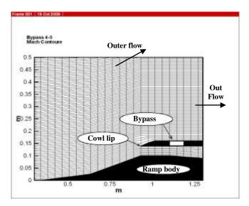
Figure (2) the air intake geometry with the types of boundaries.
