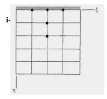
Figure (4) Grid points for lower cowl surface in computational domain.
