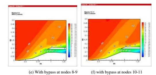
Fig ure (7) Mach Contour (a) without bypass, (b, c, d, e, and f) with bypass.
