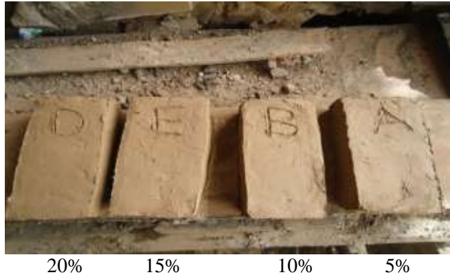
Figure (3) Samples for bricks which contain of industrial wastes( palm fiber).
