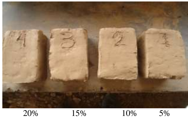
Figure (1) Samples for bricks which contain of industrial wastes ( plastic cuttings).
