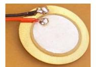
Figure (4) The piezoelectric sensor (Diameter = 15mm).
