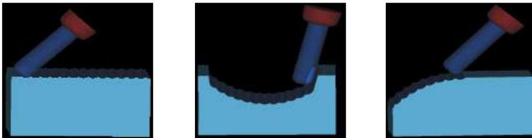
Figure (12 a, b and c). The simulation processes using UGS software for the plane, concave and convex surface respectively.
