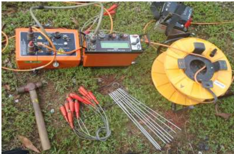
Figure (1) Tools and equipment used in electrical resistivity imaging.
