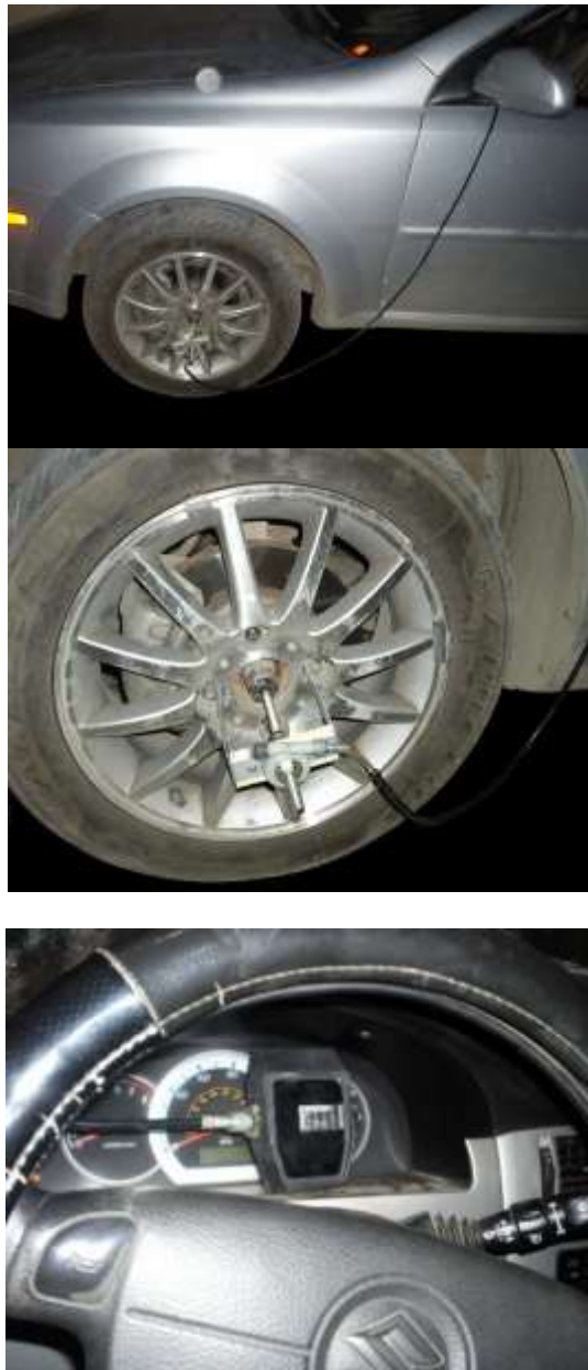
Figure (2) The wheel revolution counter mounted on the front wheel of passenger car.
