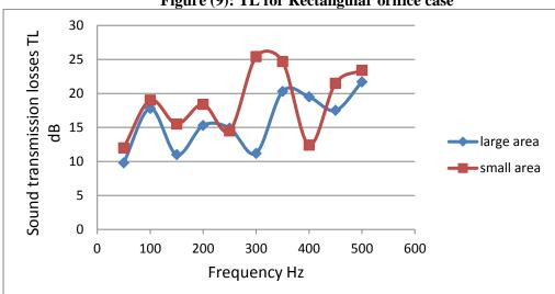
Figure (10): TL for Square orifice case
