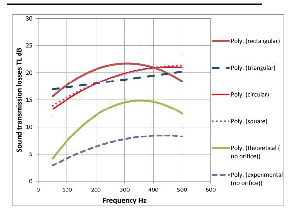
Figure (22):A comparison for the theoretical values of (TL with no orifice) and the experimental values with and without orifice.
