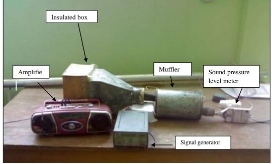
Figure (3) the test rig arrangement
