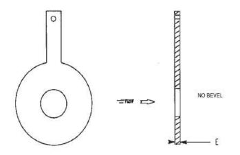
Figure (1)Restriction Orifice plate
