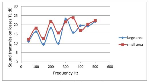
Figure (8): TL for Circular orifice case
