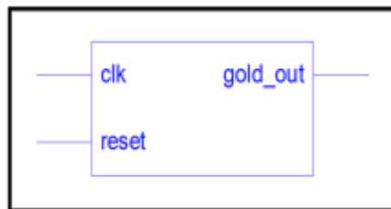
Figure (2) RTL part of Gold code generation.
