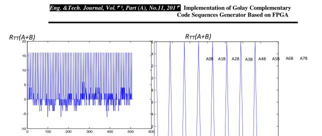
$\tau^{0^{L}}$ b Figure(3). Output of equations (3,4): a) all output for each correlation process b) only sidelobe=0 output.
