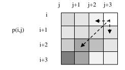
Figure (4) Boundary detection procedure: True edge if { p(i, j-1) AND p(i+1,j) AND p(i+2,j-2) } < Threshold, where Threshold  $\leq 0.35$ .
