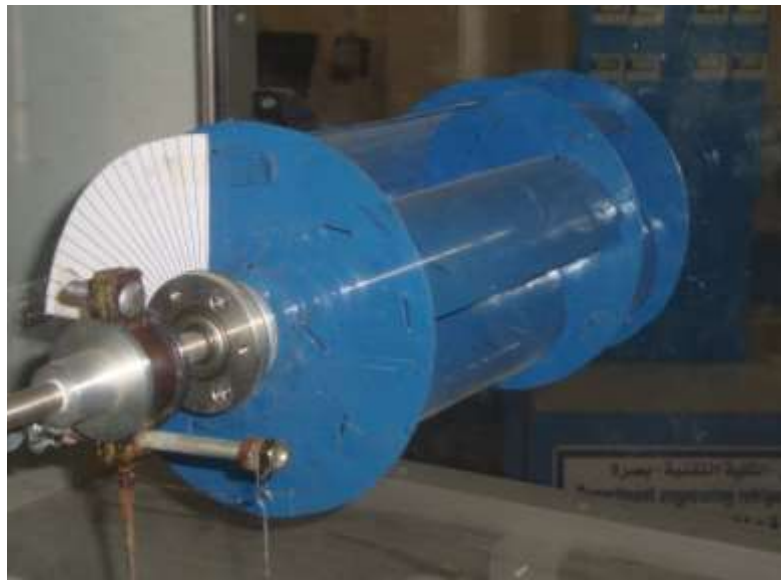
Figure (2) Savonius rotor is mounted in the wind
