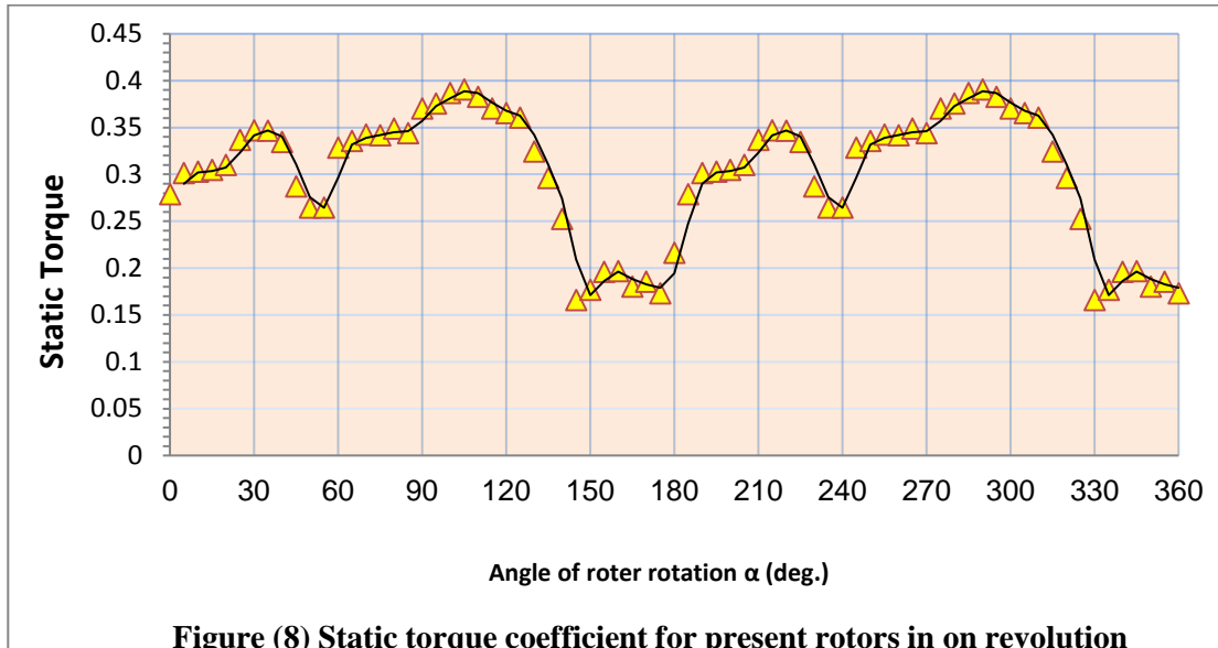
Figure (8) Static torque coefficient for present rotors in on revolution
