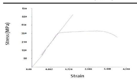
Figure (8) Stress-Strain curve for base alloy (AA 6061-T6).
