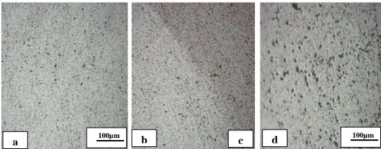
Figure (3) Microstructure of welding zones in FSW joint welded with welding parameters of (1250 rpm and 50 mm/min). a) Stir zone b) TMAZ C) HAZ d) base alloy.
