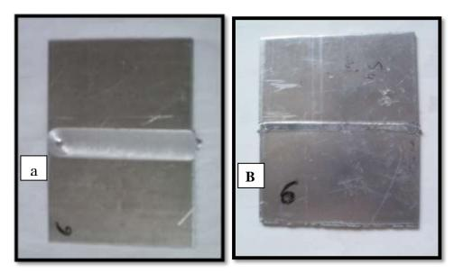
Figure (2) Configurations FSW welded plates a- The top side of butt welded plates b- The back side of butt welded plates.
