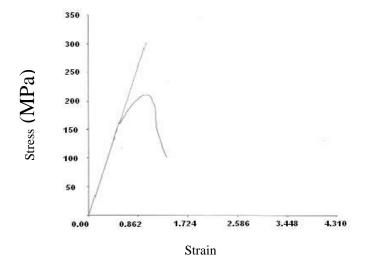
Figure (11) Stress-Strain curve for TIG joint welded at welding current 200 A.
