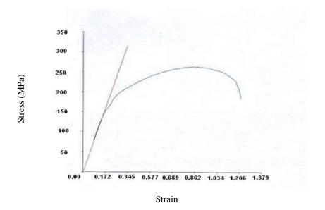
Figure (10) Stress-Strain curve for FSW joint welded at (1250 rpm50mm/min).
