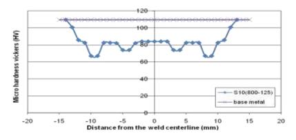
Figure (5) Microhardness profile in FSW joint welded at S10 (800 rpm-125 mm/min).
