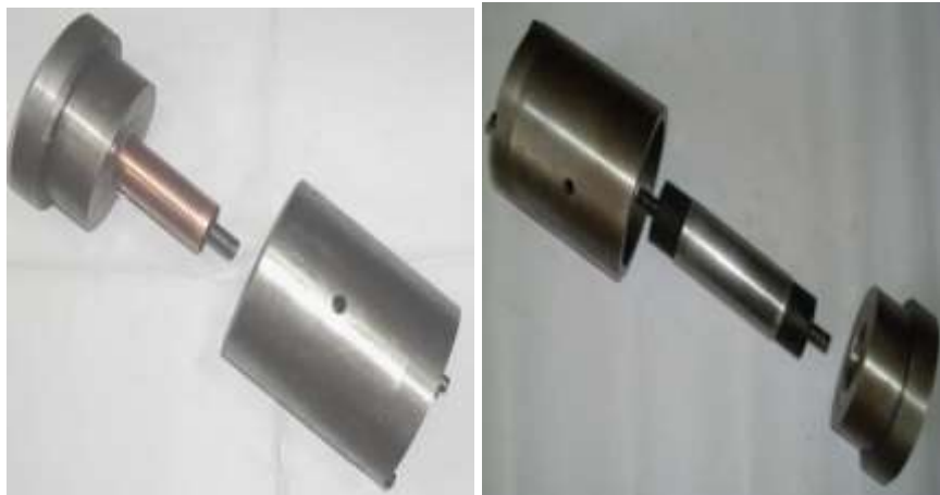
Figure (5) free bulge die for (a) Al tube (b) Cu tube.
