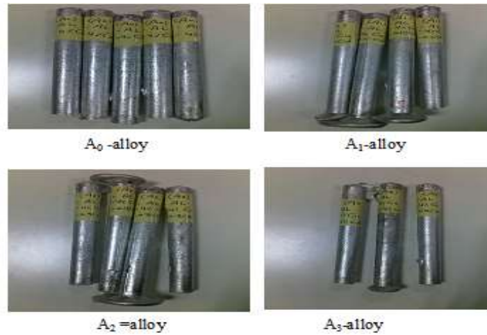
Figure (1) Samples of prepared alloys in as cast conditions.
