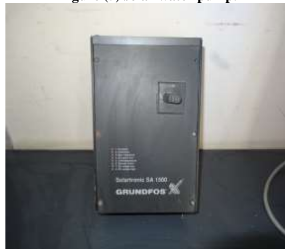
Figure (6) "Grundfos solartronic" inverter.
