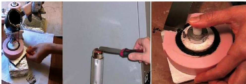
Plate (3) Pouring and Trimming of Samples.
