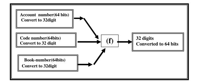
Figure (3) Inputs and Output of the proposed hash function ((f) (Operation) of proposed algorithm
