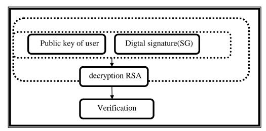
Figure(6):explain the verification process using RSA.
