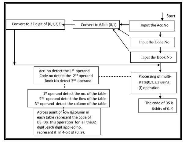
Figure(5) digital signature generation using (f)operation.
