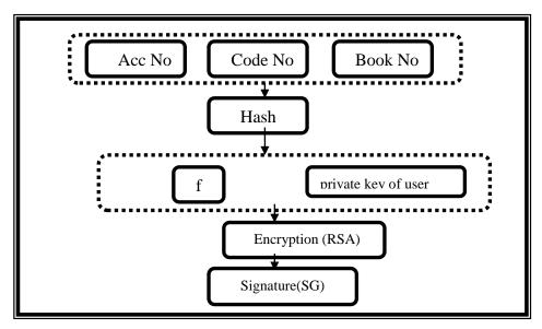
Figure(4):Explain the steps to produce the digital signature
