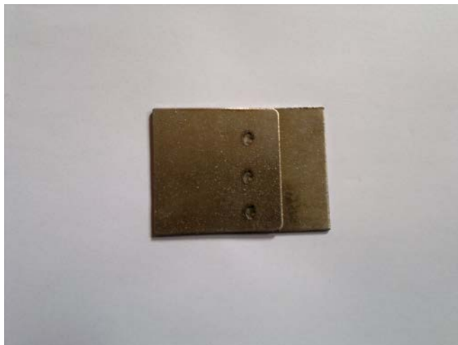
Figure (2): Plate after heat treatment, spot welding and shot peening.
