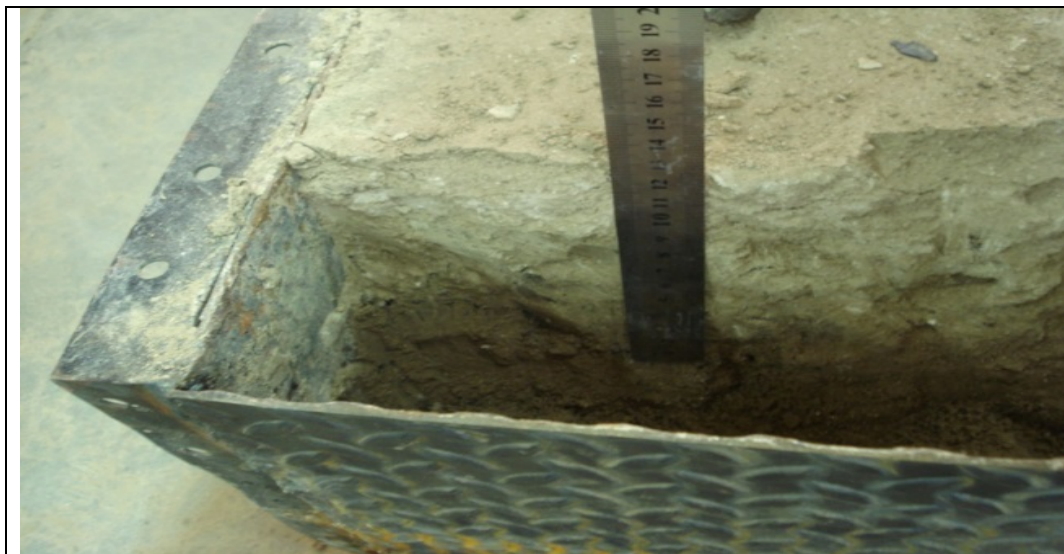
Plate (4) Effect of flow on capillary rise of water through the soil model.
