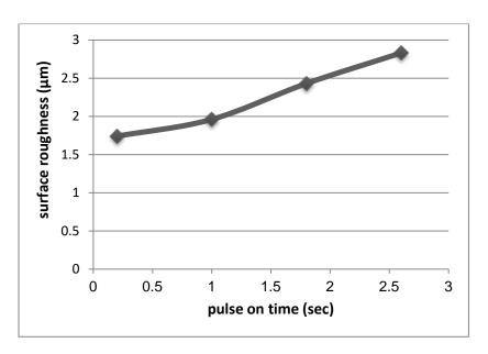
Figure (6) Effect of pulse on time on surface roughness using brass wire.
