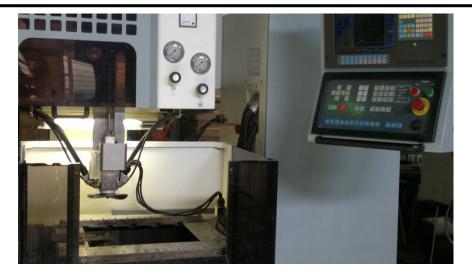
Figure (2) WEDM Cutting Machine
