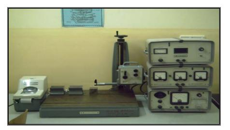
Figure (3) Talysurf4 (roughness measurements instrument)
