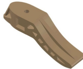
Figure (3) Final Solid Model of KEEL OF SACH Foot.
