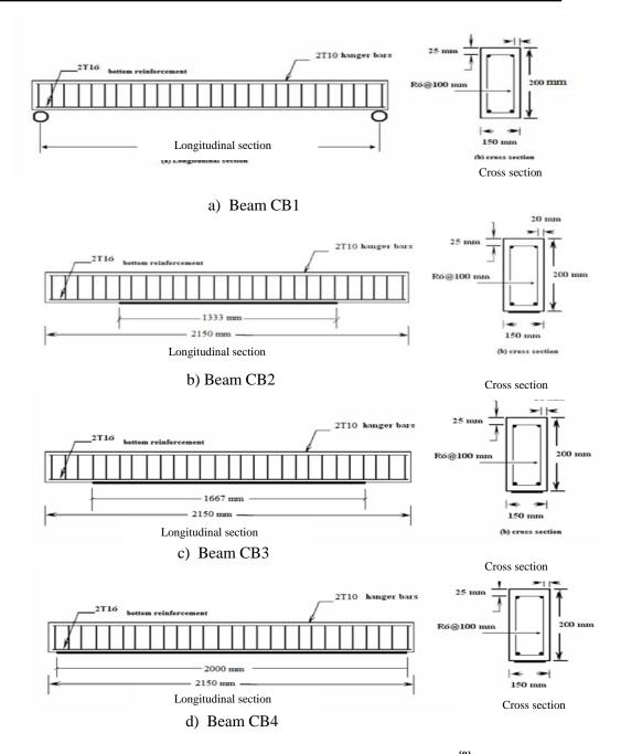
Figure (1): Geometrical properties of analyzed beams<sup>[9]</sup>.
