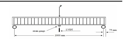
Figure (2): Loading reigns of analyzed beams<sup>[9]</sup>.
