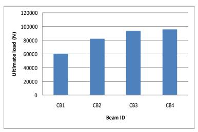
Figure(5): Ultimate loads for the analysis beams (FEM)
