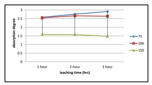
Figure (7)Effect of Leaching time on the absorption degree of alumina in AlCl<sub>3</sub> solution.
