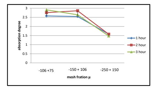
Figure (4) Effect of particle size of ore on the absorption degree of Aluminum in AlCl<sub>3</sub> solution.
