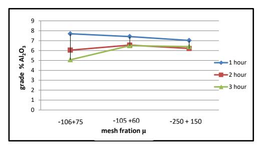
Figure (3) Effect of particle size of ore on the Alumina grade in the residual solid powder.
