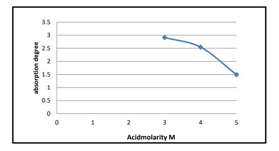
Figure (10) Effect of the acid molarity on the absorption degree inAlCl<sub>3</sub> solution.
