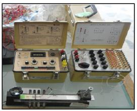
Plate (3): Calibration of the strain indicator.
