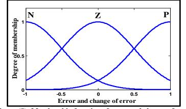
Figure (8): Membership function of error and change of error
