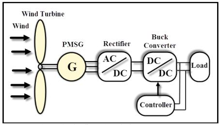
Figure (2): Configuration of wind energy system
