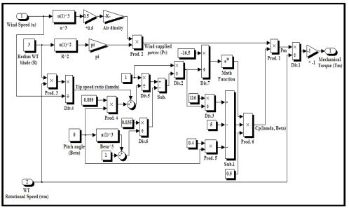
Figure (4): Simulink model of the wind turbine
