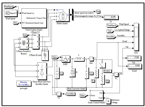
Figure (9): Simulink model of wind energy system
