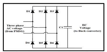
Figure (6): Three-phase full bridge rectifier
