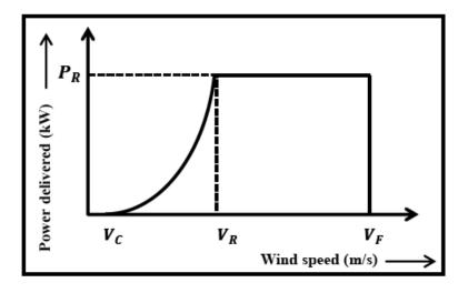
Figure(1) : Typical curve of a wind turbine
