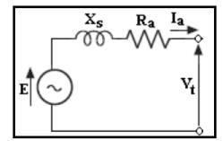
Figure (5): Equivalent circuit of PMSG for one phase
