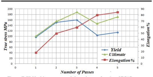
Figure (7) Yield, ultimate stress and elongation as a function of ECAR passes.
