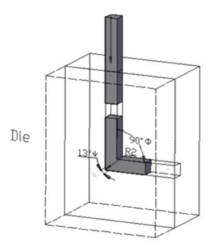
Figure (1) a scheme of the ECAP die
