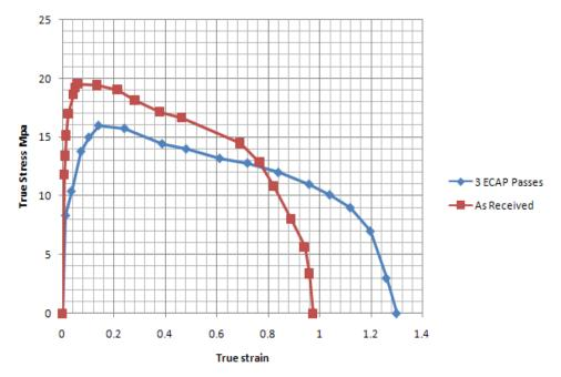
Figure (13) True stress true strain curve for the as received and 3pasess ECAP at strain rate of  $2.45 \times 10^{-4}$  s<sup>-1</sup> and temperature of 623 K.
