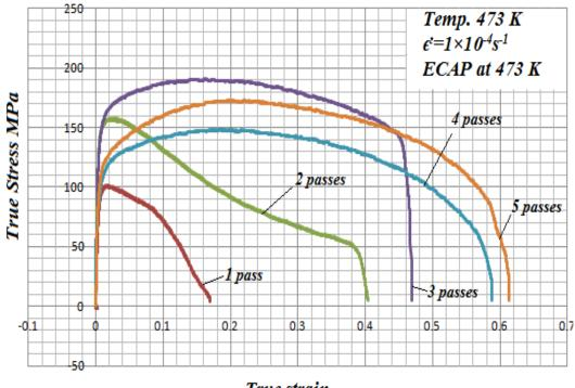
*True strain* Figure (6) stress strain curves for specimens made from the ECAP billet
