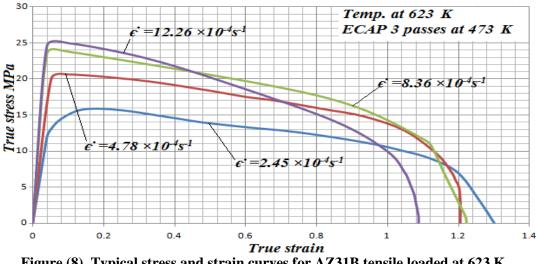
Figure (8) Typical stress and strain curves for AZ31B tensile loaded at 623 K
