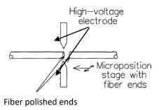
Figure (1): Fusion splicing technique.
