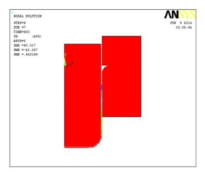
Figure (1) Finite element model of the sheet material and drawing die
