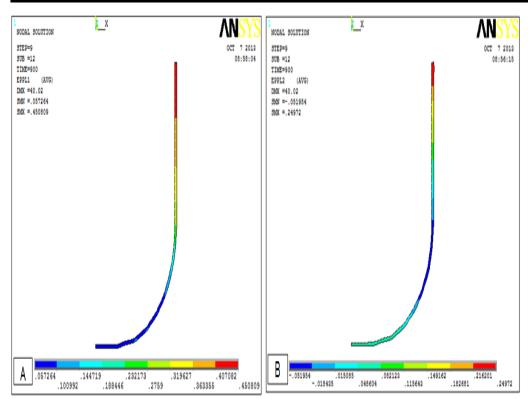
Figure (2) The strain distribution on cup wall of tool geometry, (A) radial strain, (B) thickness strain
