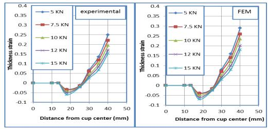
Figure (8) Effect of blank holder force on thickness strain
