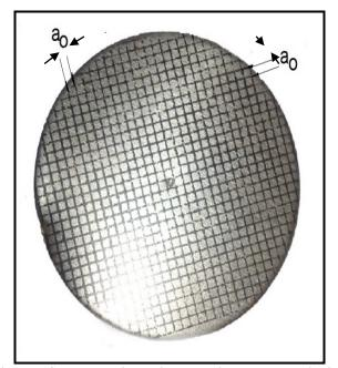
Figure (4) Blank with grid, by using screen printing
