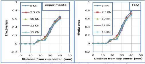
Figure (10) Effect of blank holder force on effective strain
