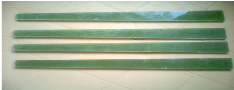
Figure (2): Laminated tapered beam specimens.
