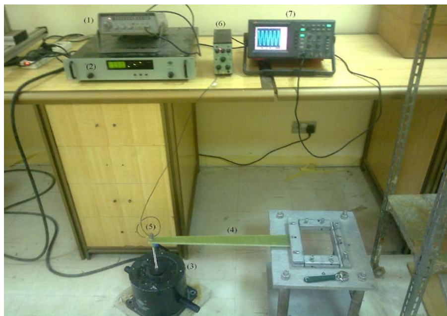
Figure (3): Experimental set up for modal testing of a laminated cantilever blade. (1) Signal generator (2) Power amplifier (3) Electro dynamic exciter (4) Test beam (5) Accelerometer (6) Charge amplifier (7) Oscilloscope.
