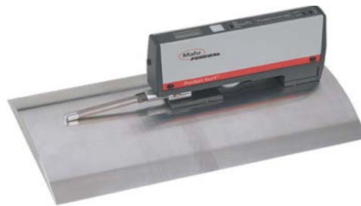
Figure (4) Surface roughness measurement
