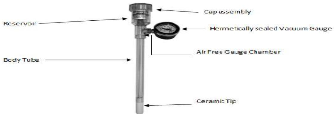
Plate (4): IRROMETER (IRROMETER Manual Book, IRROMETER company, Inc.)
