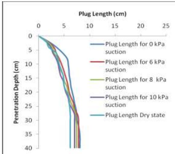
Figure (7): Average soil plug length for group of triple pipe piles of 40 cm long pressed in different state soil (dry, full saturation and unsaturation with average matric suction 6, 8 and 10 kPa ).
