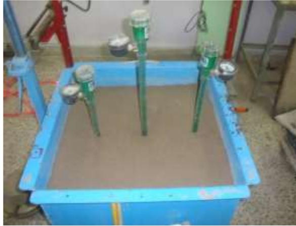
**Plate (5): Inserting three Tenseometers for profile set suction**
