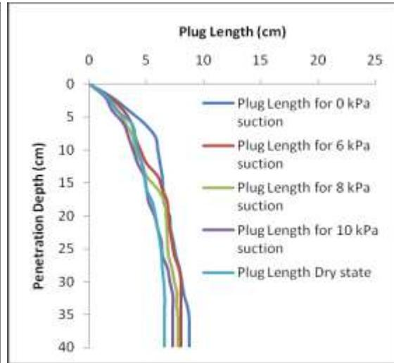
Figure (6): Average soil plug length for group of double pipe piles of 40 cm long pressed in different state soil (dry, full saturation and unsaturation with average matric suction 6, 8 and 10 kPa ).
