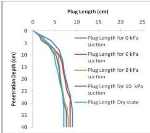
Figure (5): Average soil plug length for single pipe pile of 40 cm long pressed in different state soil (dry, full saturation and unsaturation with average matric suction (6, 8 and 10 kPa).
