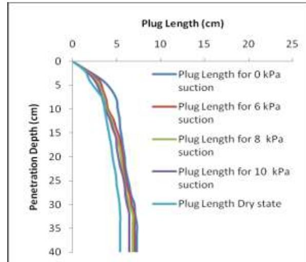
Figure (8): Average soil plug length for group of six pipe piles of 40 cm long pressed in different state soil (dry, full saturation and unsaturation with average matric suction 6, 8 and 10 kPa ).
