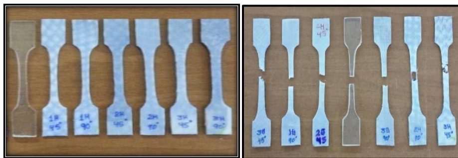
Figure (3): Samples of prosthetic pylon specimens before and after tensile test.
