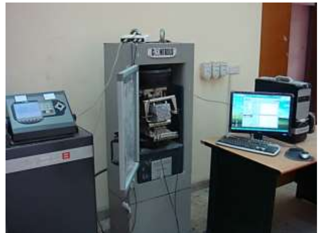
Plate 2: The apparatus used to conduct the modulus of rupture test
