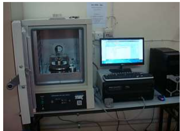
Plate 3: The apparatus used to conduct the thermal conductivity test
