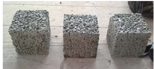
Plate 1: No-fines concrete samples used in the test of compressive strength
