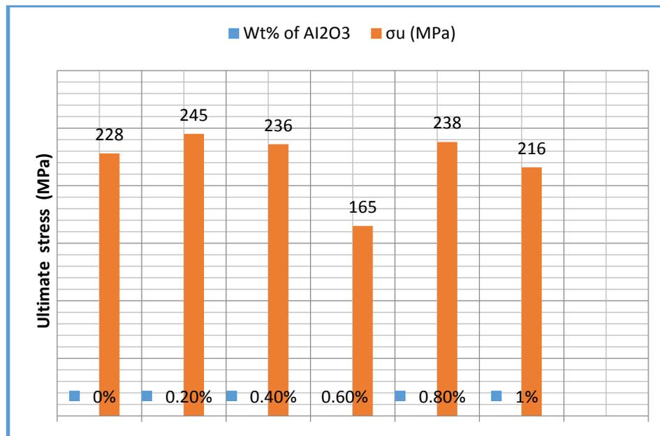
Figure 3: Variation of Ultimate tensile strength against Al<sub>2</sub>O<sub>3</sub> wt %
