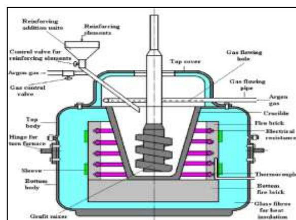
Figure 1: X Manifesting device for manufacturing the MMC<sub>s</sub> composites
