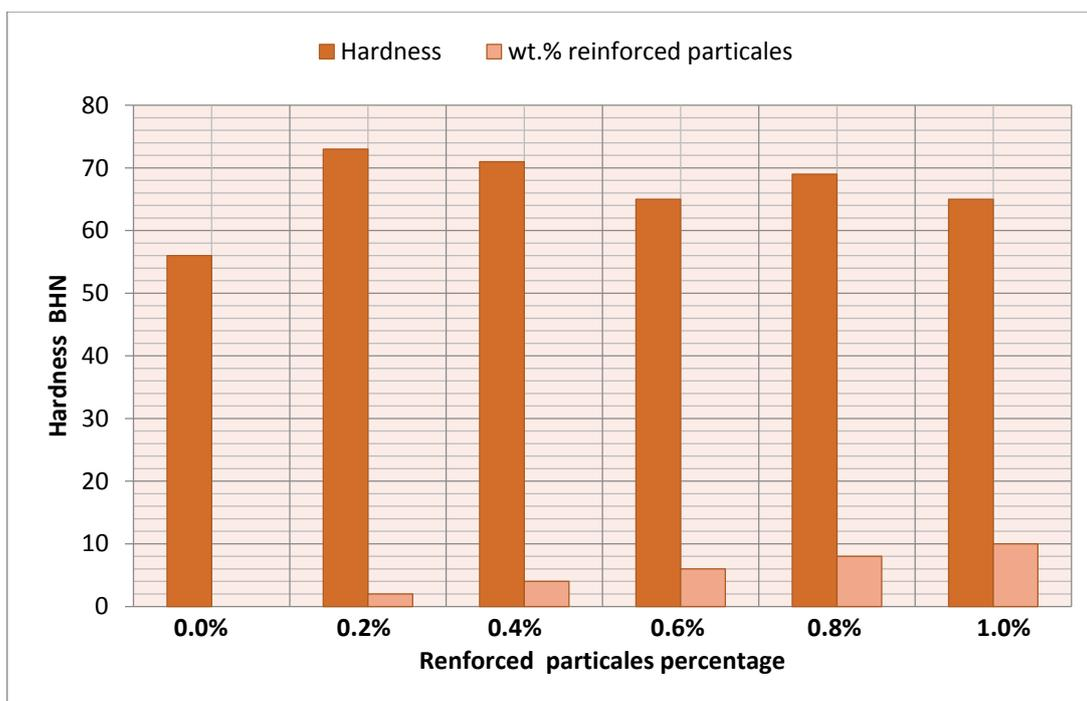
**Figure 2: Hardness (BHN) against Al<sub>2</sub>O<sub>3</sub> wt% , average of three attempt testing**
