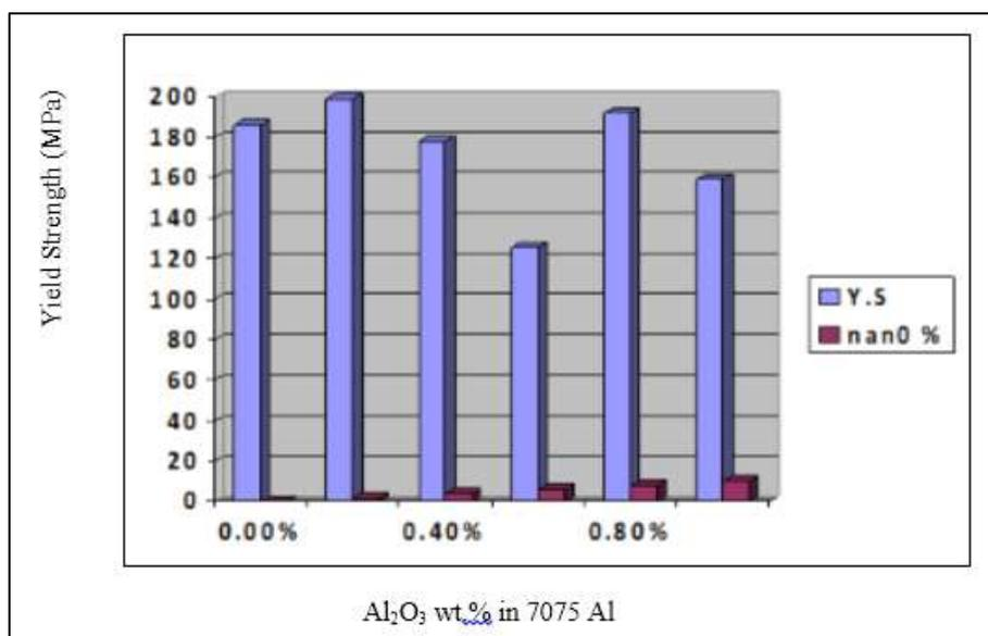
Figure 4: Yield strength of MMCs composite against wt% of Al<sub>2</sub>O<sub>3</sub> in 7075 Al
