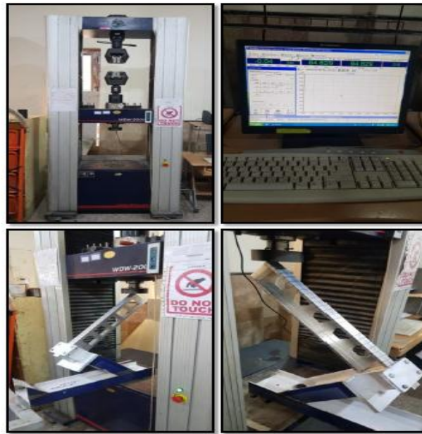
Figure 6: Buckling test under combined loading
