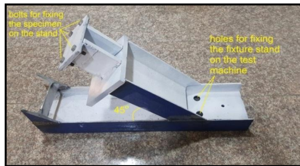
Figure 5: the fixture stand of test specimens
