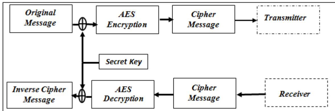
Figure 3: Encryption / Decryption by AES [16]
