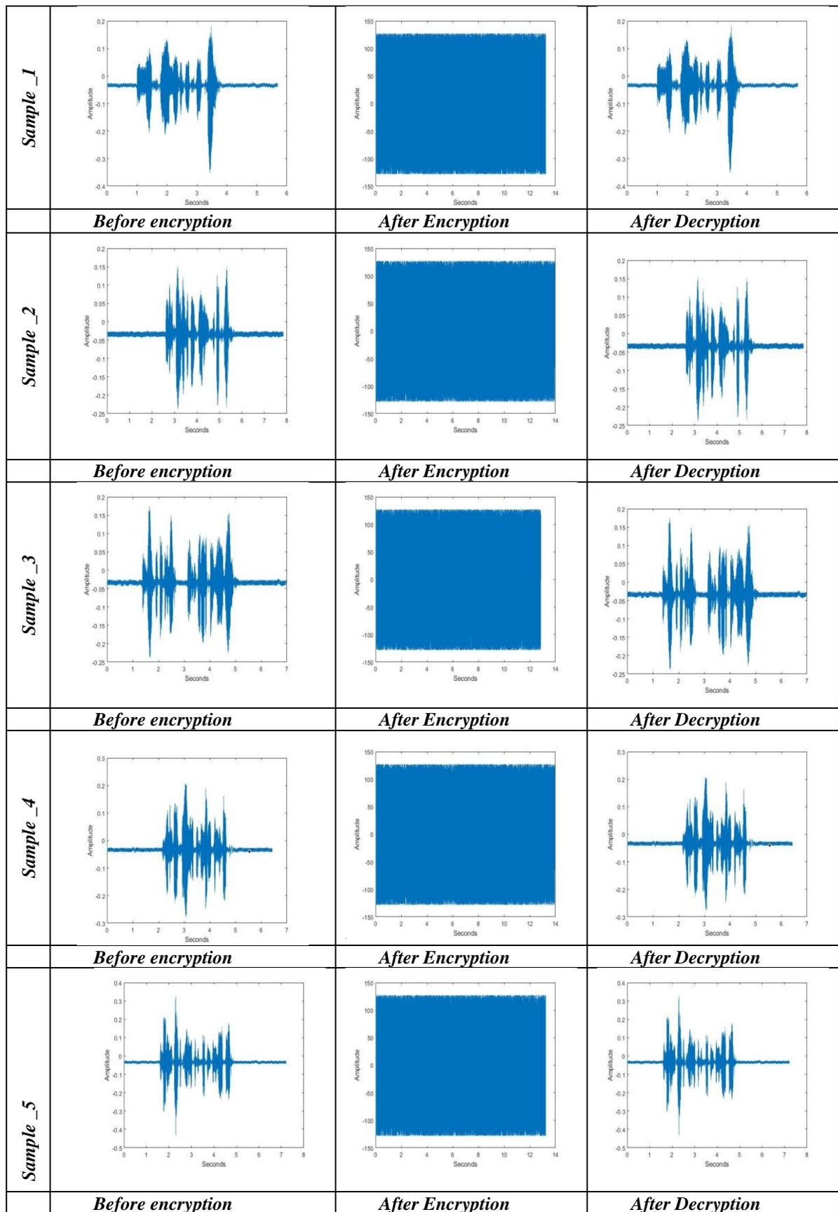
**Figure 6: Shows a Waveform of an Original, Encryption and Decryption Voice Signals**
