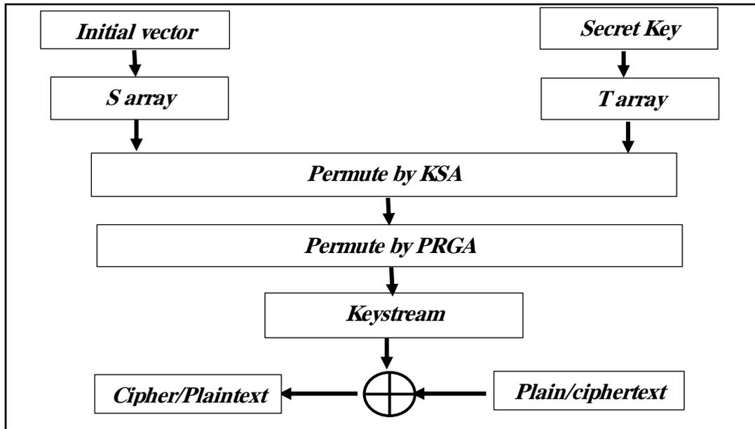
Figure 2: Encryption / Decryption by RC4 [13]
