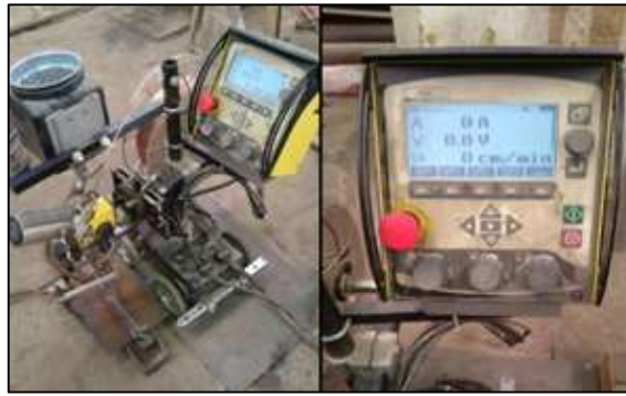
Figure 2: EsabA2 Multitrack with the A2-A6 process controller PEK
