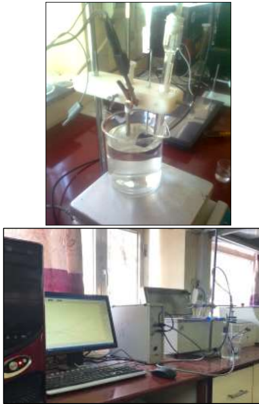
Figure 4: The used setup for the electrochemical measurements
