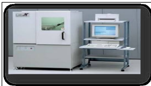
Figure 6: X-ray diffraction device of residual stresses measuring
