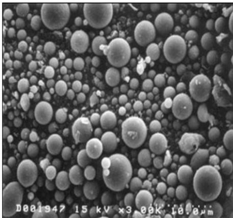
**Figure 2: SEM of (FA) particles at 2000X [24]**
