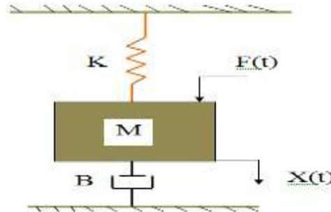
Figure 4: Simulated model for the pipeline liquid [1]
