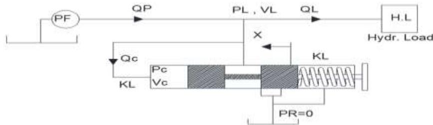
Figure 3: Single-stage pressure control relief valve
