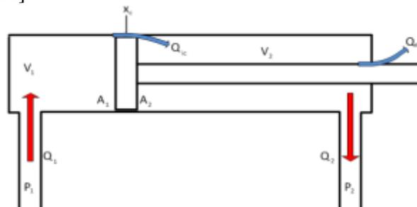
**Figure 2: Schematic diagram of a double-acting cylinder [13]**
