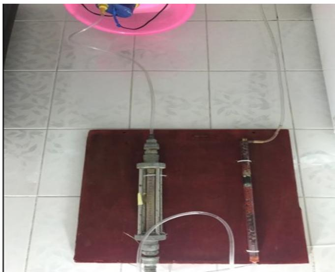
Figure 3: show the packed bed reactor
