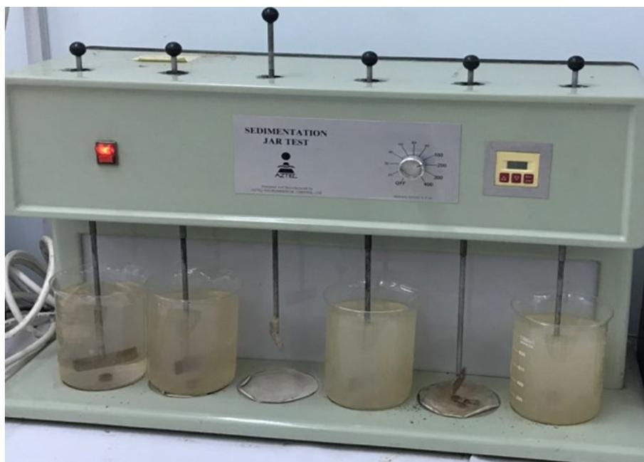
Figure 1: show the beakers in the jar test instrument
