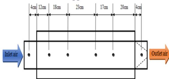
Figure 3: Thermal sensor distribution network on design
