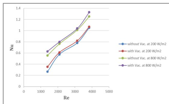
**Figure 12: The amounts of Nusselt number with an adapted Reynold number for different irradiance with and without vacuum**
