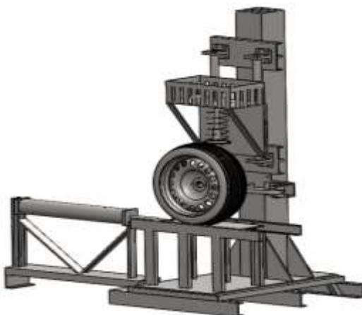
Figure 1: Quarter Car Test Rig
