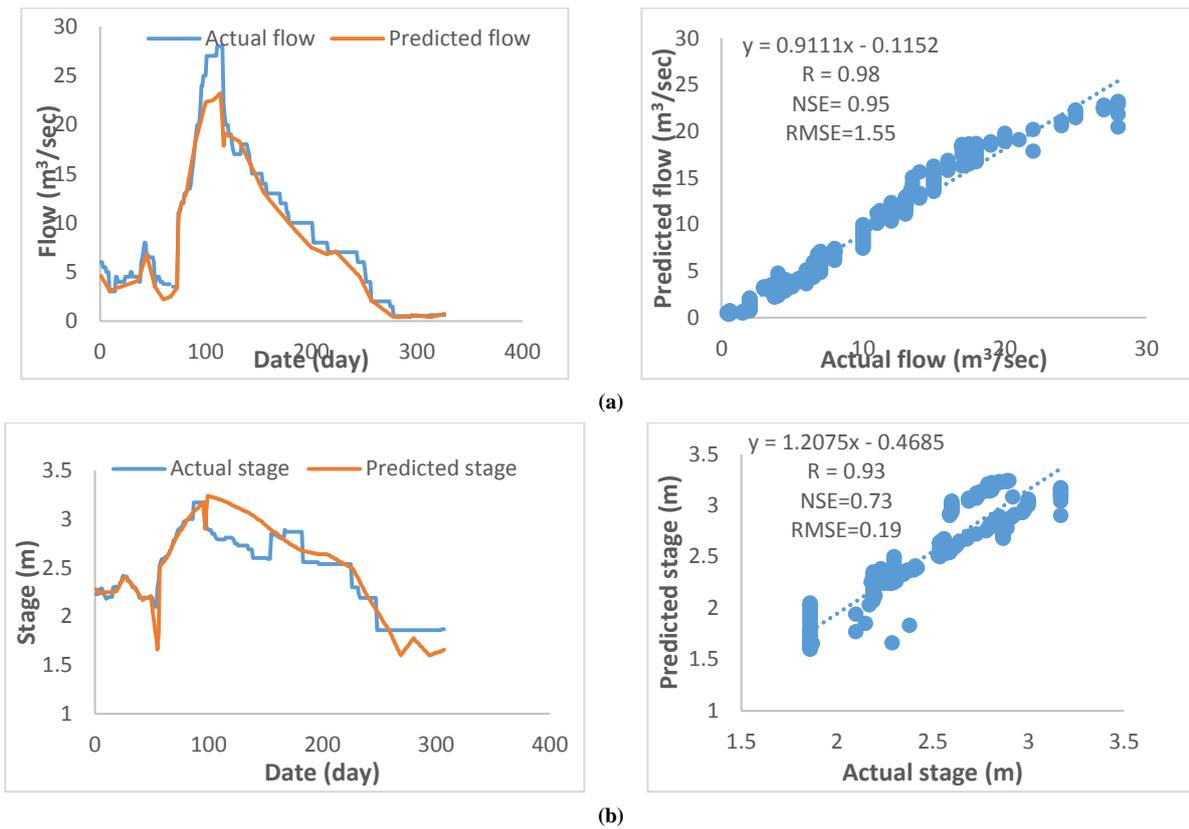
Figure 3: Comparative plots of observed and predicted flow in Abu-Ziriq Marsh using HEC-DSSVue for (a) flow and (b) stage
