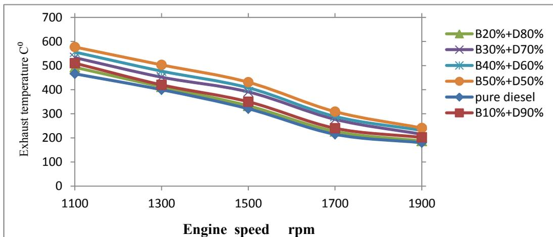
Figure 6 : Variation of exhaust temperature with engine speed
