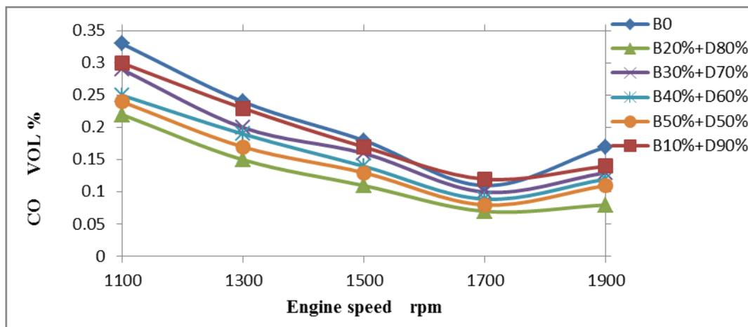
Figure 9 : Variation CO emission with engine speed.
