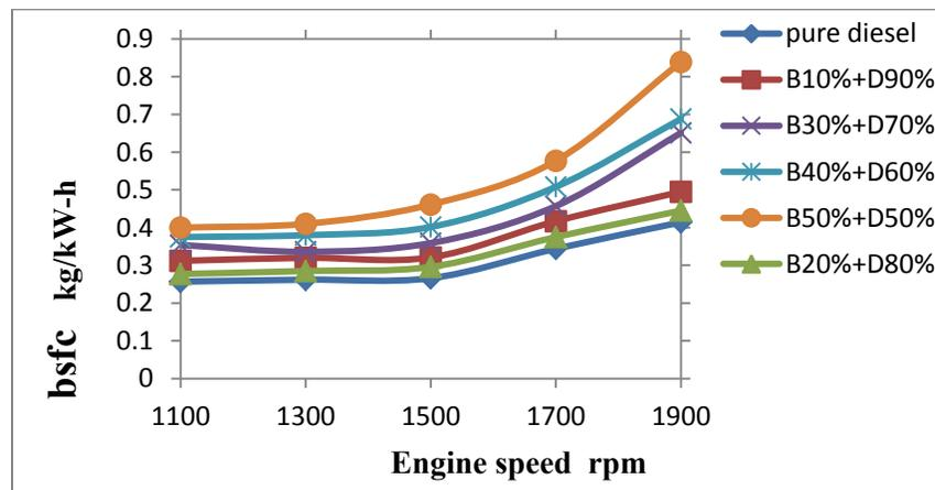
Figure 4: Change the BSFC with engine speed rpm.
