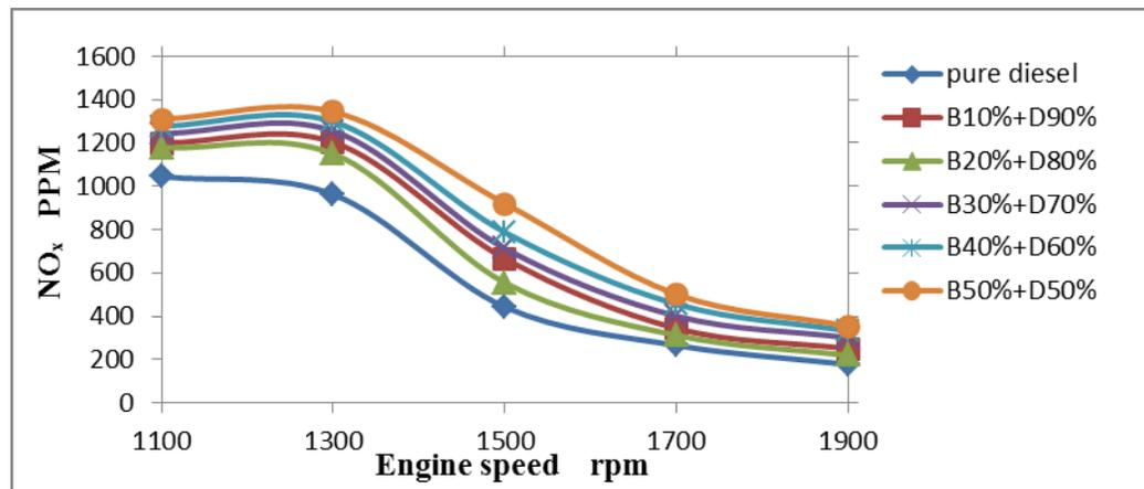
Figure 8 : Variation NO<sub>x</sub> emission with engine speed
