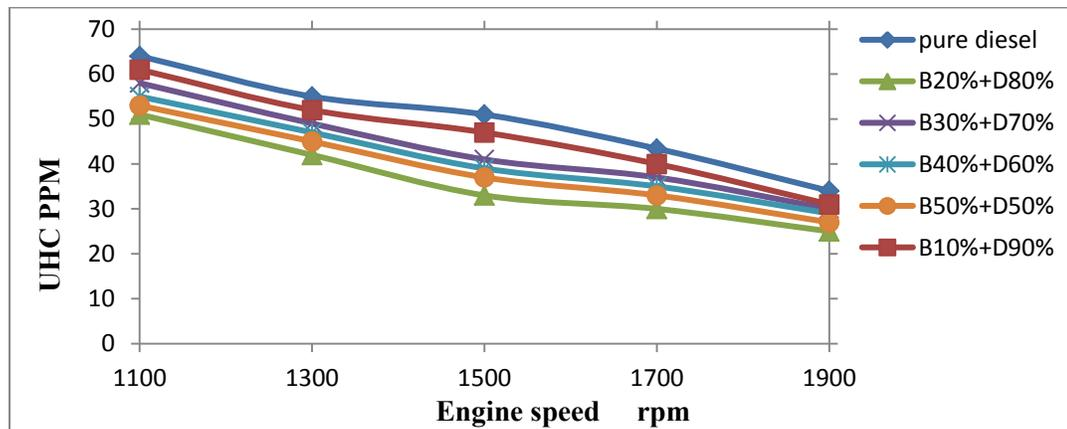
Figure 7 : Variation of UHC with engine speed
