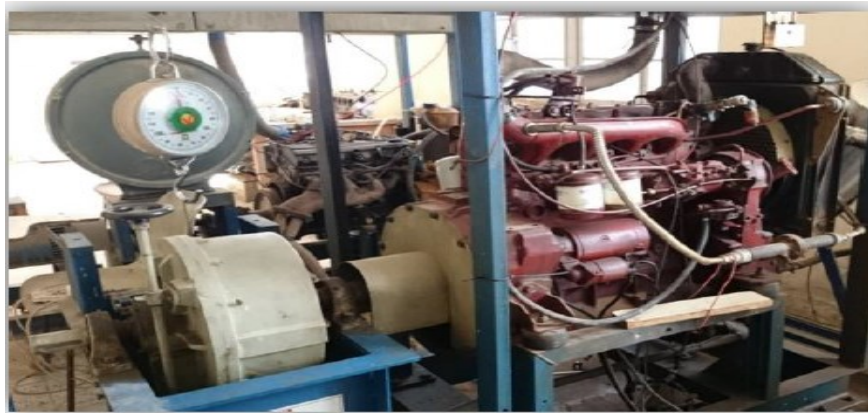
Figure 1: The FIAT Diesel engine with dynamomete
