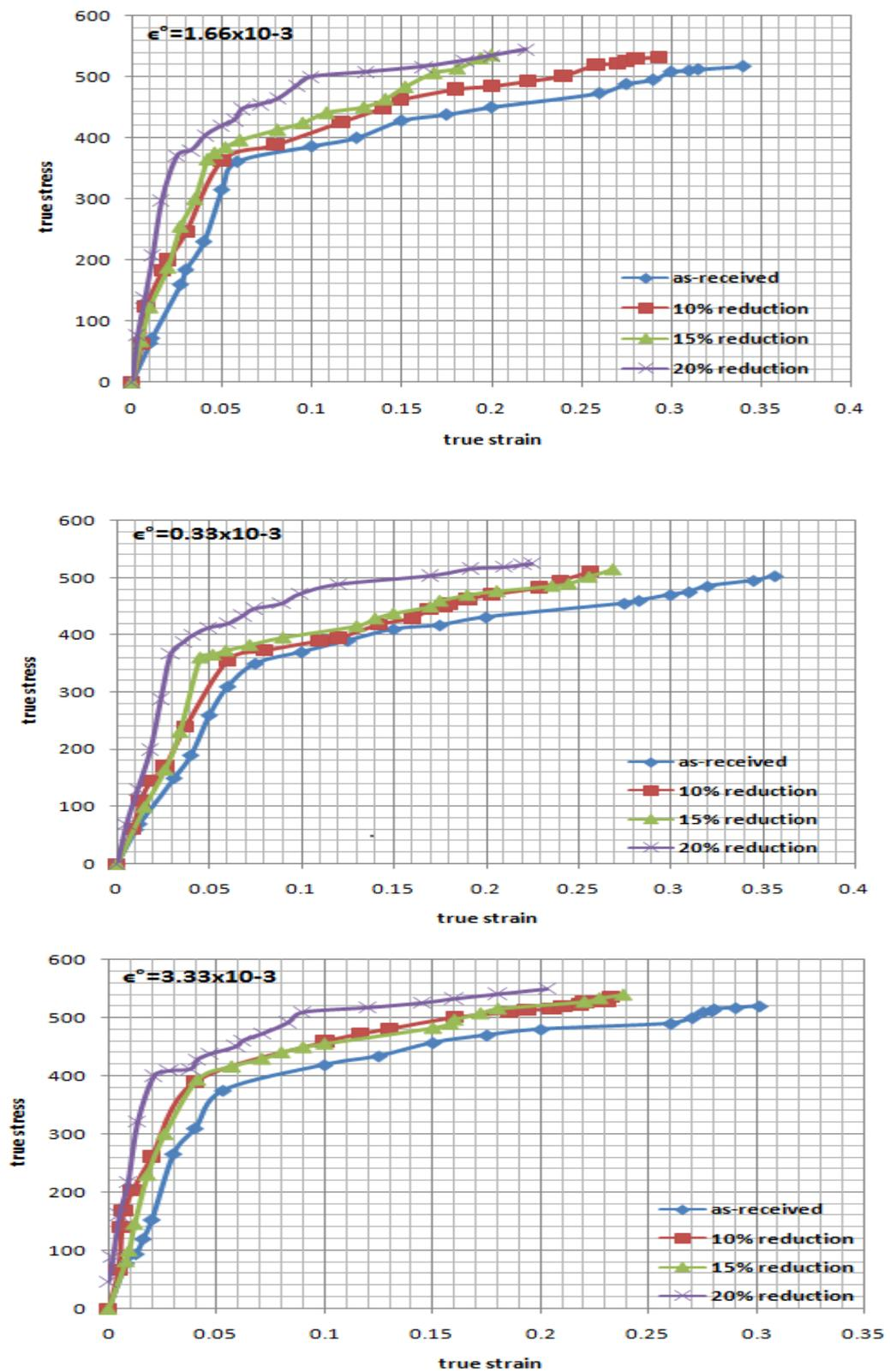
Figure 7: True stress-strain curves of tensile test for different ASRed specimens and constant initial strain rate  $0.33 \times 10^{-3} s^{-1}$ ,  $1.66 \times 10^{-3} s^{-1}$ ,  $3.33 \times 10^{-3} s^{-1}$  respectively
