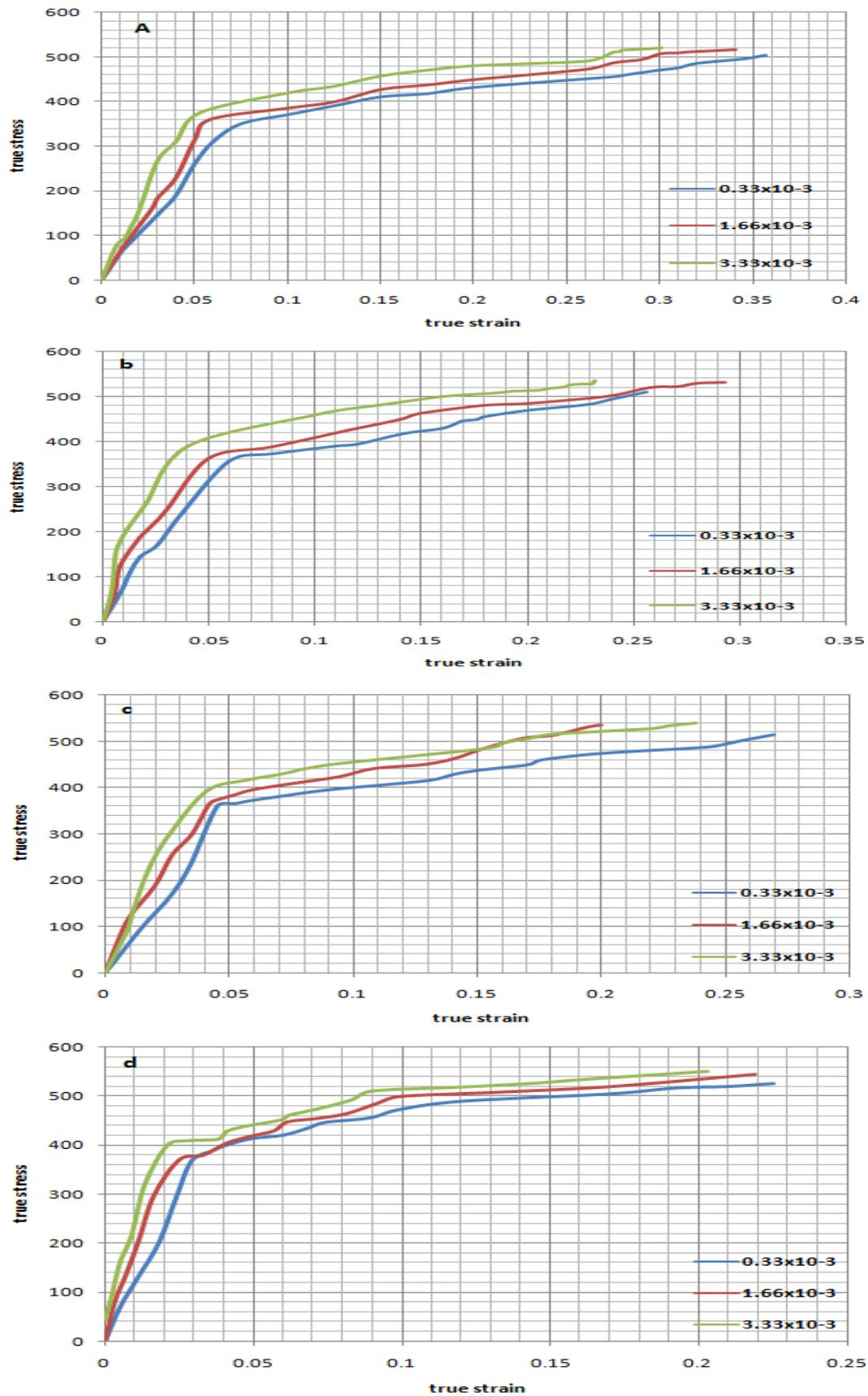
Figure 6: True stress-strain curves of the tensile test at different initial strain rates for 2024-T351 specimens (a) As-received (b) 10% thickness reduction (c) 15% thickness reduction (d) 20% thickness reduction
