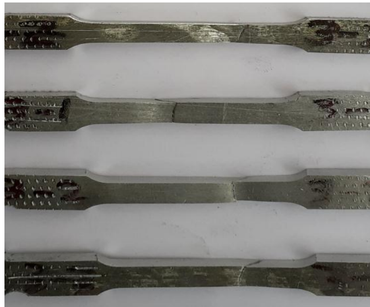
Figure 5: Image illustrated of the specimens after the tensile test
